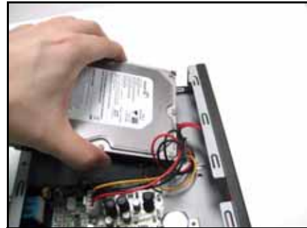
Figure 27.5 Insert the drive carefully
